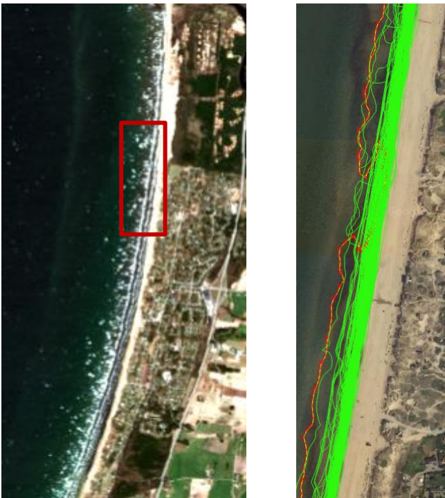
Figure 18: Acquisition during strong winds (left, RGB S2 image) leads to wrong shoreline extraction (red line in the right image)
