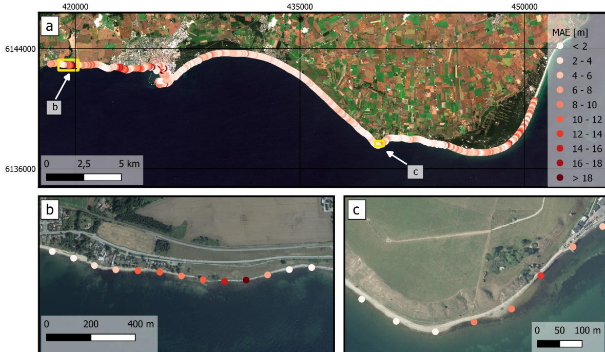
Figure 6: Spatial distribution of MAE for the co-registered SDS along the coast of Ystad municipality. Yellow boxes in A show the positions of subsets B and C. B: Differences of MAE at the sandy and rocky parts of the beach near Svarte. C: MAE south of Kåseberga. Background image in A is the Sentinel-2 MSI RGB from 20.07.2021, whereas the orthophoto from 2020 provided by Swedish Land Survey was used as background in B and C.
